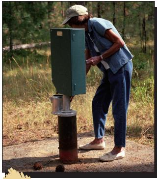
Figure 71—This accessible handpump is operated by a crank, making it possible for almost everyone to draw water independently.
